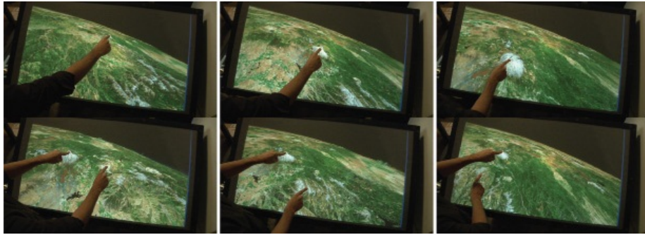
Figure 2.11: The screen-space direct manipulation interaction technique interaction in two scenarios for interacting with a globe. The top scenario moves the mountain closer with a one-touch movement, whereas the bottom scenario moves the mountain further away and rotates the earth around the mountain at the same time (image from [Reisman et al., 2009]).
