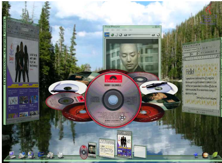
Figure 2.14: Project Looking Glass: a 3D window manager, allowing 3D placement of windows, writing notes on the back of windows, and 3D objects to be used in the window manager.
