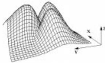
Fig. 1. 3D surface of blended Gaussian curves
