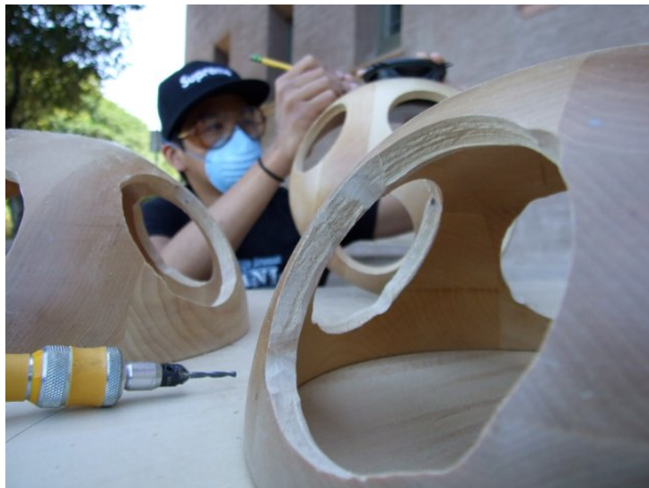
Figure 2.11: Making speakers from salad bowls. The holes are for mounting car speaker drivers. [115]
