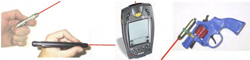
Figure 8: Laser pointer devices used in a comparison between remote pointing, direct-touch and 2D mouse input [Myers et al., 2002] (from left to right): conventional laser pointer, pen-like laser pointer, pda-mounted, and toy gun mounted laser pointer.
