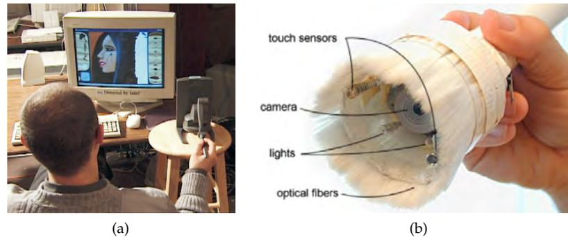
Figure 1: Parts of the DAB [Baxter et al., 2001] and I/O BRUSH [Ryokai et al., 2004] user interfaces: a SensAble Phantom with haptic feedback for desktop use (a) and a physical brush equipped with camera, light, and touch sensors for capturing real world textures (b).
