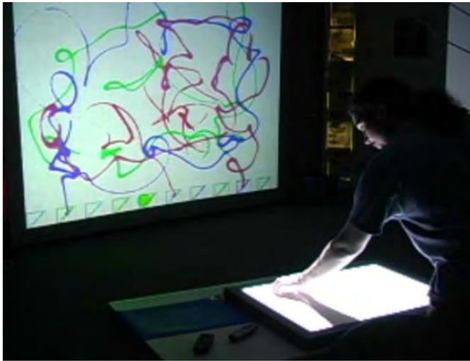
Figure 3: In 3D fluid Jet Painting [Lee et al., 2006] the user interacts with a virtual paint bucket on a Diamond-Touch table. The resulting image is projected on a wall mounted display.
