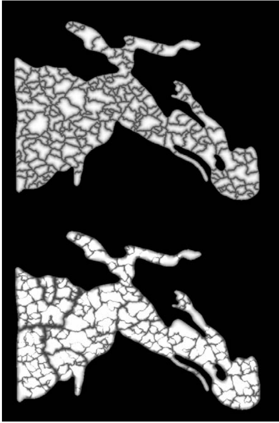
Figure 6: Crack before (top) and after (bottom) aging and widening due to T-junctions.
